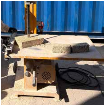
Cutting Biomattone® with a band saw
